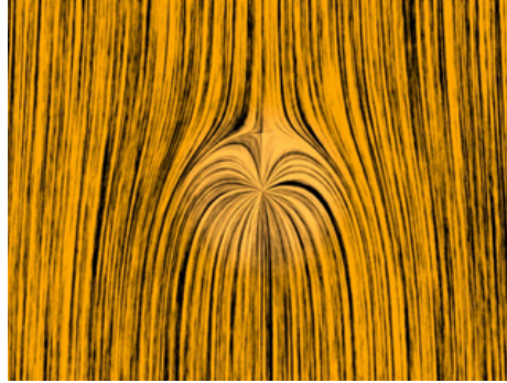
Figure 1.4.4 A constant downward flow interacting with a diverging flow (source). In the language of vector calculus, we represent the flow field of a fluid by
