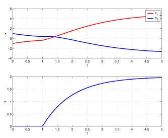
State variables of the system and its output for  $x(0) = \begin{bmatrix} 4 & -4 \end{bmatrix}^T$
