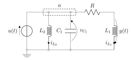
The input of the system is the u(t) current and the output of the system is the y(t) voltage drop across the  $L_1$  inductor.
