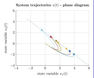
Figure 1. Simulation of system (7) from different initial conditions  $x(0) \in x_0 + \text{Ker}(\mathcal{O}_2)$  (denoted by dots) with zero input. As one can observe, the state trajectories are different, however this difference does not appear in the output of the system. In this example  $u \equiv 0$  and  $x_0 = \begin{pmatrix} 1 \\ 1 \end{pmatrix}$ . The blue dashed line in the right figure illustrates the actual unobservability subspace of the system corresponding to  $x_0$ .
