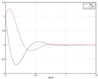
$$u_C(0) = 1 \text{ V}, i(0) = 1 \text{ A}, u_{be}(t) = 5 \text{ V}$$
