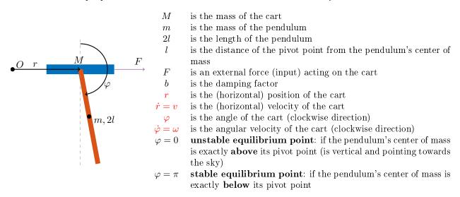
This system has a nonlinear equation, which can be linearized in a certain operating point (see Appendix). The state vector of the system is the following:  $x = \begin{pmatrix} r & v & \varphi & \omega \end{pmatrix}^T$ , furthermore, the external force F constitutes the input of the system (u). The nonlinear model of the system is:  $\dot{x} = f(x) + g(x)u$ , where
